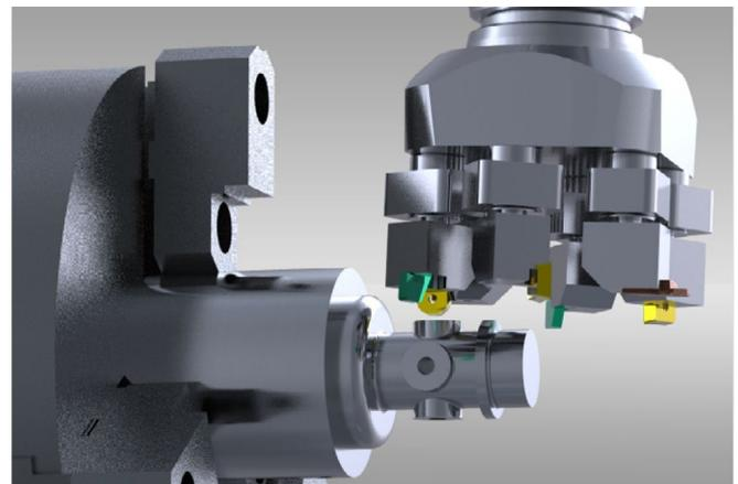
Turning in PTC Creo Production Machining.
