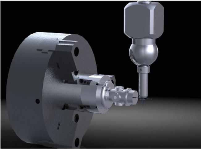
For production machining applications, PTC Creo complete machining improves manufacturing set-up and quality control processes with in-process probing support.
