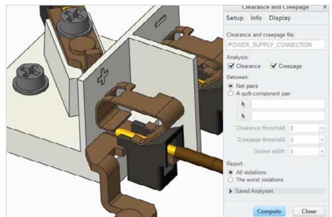
PTC Creo Spark Analysis Extension helps you automate electrical clearance and creepage analyses of 3D designs.
